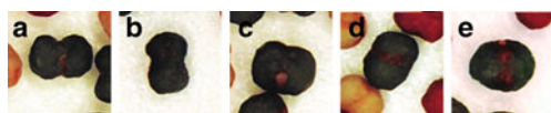
Fig. 7. Images of pellets (pure CAR) using different water contents 240% (left, a), 264%, 288%, 312%, and 336% (right, e) after 5 min spheronization
