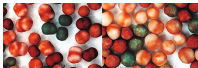
Fig. 2. Pellets obtained from MCC ( left , water content 151%) and MCC-lactose ( right , water content, 74%) after 5 min spheronization
