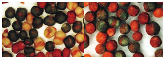
Fig. 3. Pellets obtained from CAR ( left , water content, 312%) and CAR-lactose ( right , water content, 152%) after 5 min spheronization
